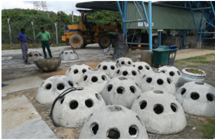
Ready Mix Concrete samples discarded in the quality testing process are upcycled to make the Reef Balls used for coral replanting
