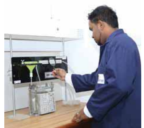
Concrete Initial Surface Absorption Testing
